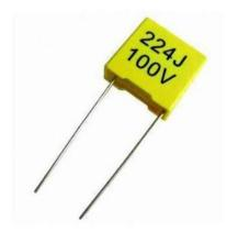
The value might be either shown in an explicit way either on the side, or on the top of the component, or like the ceramic capacitors. For instance, 220n stands for 220 nF. The value 224 means 220nF as well. Sometimes, instead of 1.5n, you might find 1n5. In other words, the decimal place is removed and changed with the multiplication factor (typically n).
