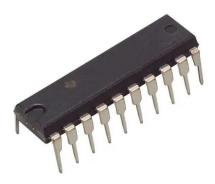
In our kit you will either find 3-terminal voltage regulators (they have the same package of transistors) or dualin line package (DIP). ICs have a specific orientation which is shown either by a dot, or by a "D" slot.
