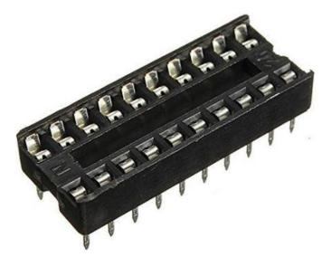
Of course, you must first solder the IC socket (pay attention to the notch, to match the IC pin 1 indicator!), and then, once you have finished soldering all the components, you can insert the IC.
