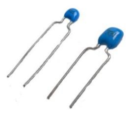
The capacitance value is shown numerically, but not explicitly: the value is encoded in a similar way used for resistors. That is, the first two digit make the numerical value of the capacitor, and the third digit shows how many zeroes you must add to the right of the first two numbers. The final number you get is the capacitance in PicoFarad ( $10^{-12}$  F)
