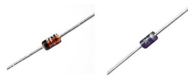
Diodes are polarized devices, and must be inserted correctly. In particular, there is always one band close to one of the two terminals, which indicates the cathode. The diode should be placed with the band as indicated in the silkscreen.
